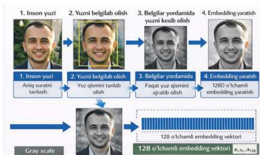
4-rasm. Inson yuzidan 128 o‘lchamli vektorga aylantirish.
